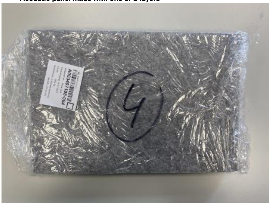
Picture 1: Acoustic panel made with one or 2 layers
