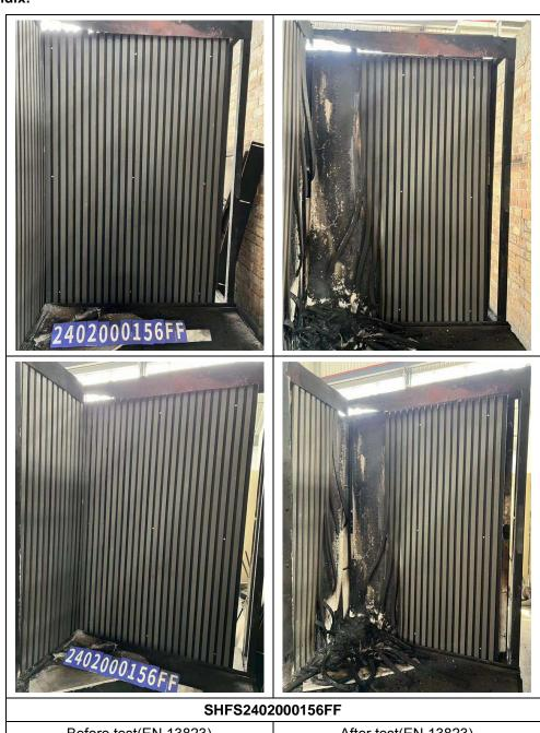
Before test(EN 13823) After test(EN 13823)
